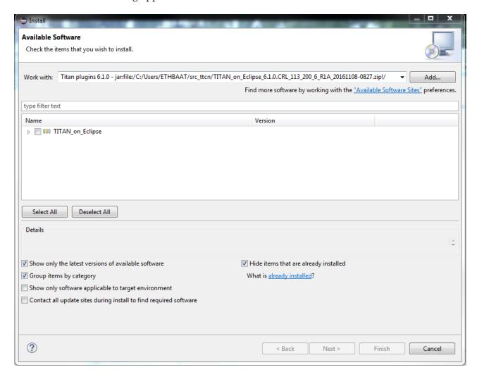
4. It is advised to uncheck the "Contact all update sites..." box. Select the TITAN plug-ins and the external dependency plugins to be installed.
