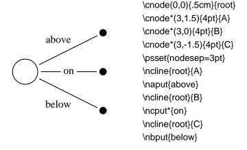
**\naput** and **\nbput** use the same algorithm as **\uput** for displacing the labels, and the distance beteen the line and labels is **labelsep** (at least if the lines are straight).
